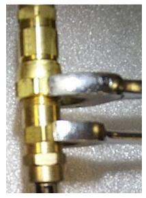
REMOVE THE PROTECTIVE PLASTIC CAPS FROM THE MALE AND FEMALE FITTINGS TO BE CONNECTED. BE SURE BOTH FITTINGS ARE CLEAN BEFORE ASSEMBLING. FINGER TIGHTEN, TURNING THE LARGER FITTING UNTIL SNUG.
