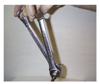
HOLD THE 5/8" FITTING WITH THE WRENCH AND FURTHER TIGHTEN THE 3/4" FITTING AS SHOWN AT THE LEFT.
